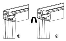
e. Tear the cords. Put the buckle bead into groove of headrail end cap (make sure the bead buckle from groove top down) as drawing.
